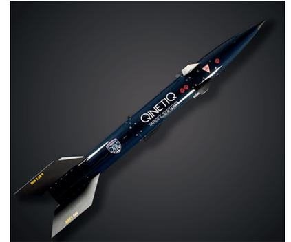
The GAL-ST transmits Time Space and Positioning Information (TSPI) and target status telemetry data in real time for range safety and operational requirements monitoring, and can accommodate radar or infrared augmentation, and other payload integration for specific weapon system requirements. Additionally, the target includes a Flight Termination System to maintain range safety during all phases of flight.
