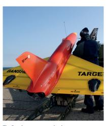
The Banshee target can simulate an enemy aircraft or cruise missile
