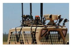
Any Bobcat Loader equipped with Bobcat's Selectable Joystick Controls can be transformed into a high performance robotic platform using QinetiQ's RAK mounting system.
