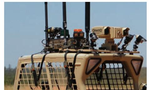
Any Bobcat Loader equipped with Bobcat's Selectable Joystick Controls can be transformed into a high performance robotic platform using QinetiQ's RAK mounting system.
