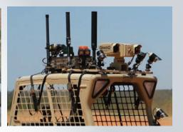
Any Bobcat Loader equipped with Bobcat's Selectable Joystick Controls can be transformed into a high performance robotic platform using QinetiQ's RAK mounting system.
