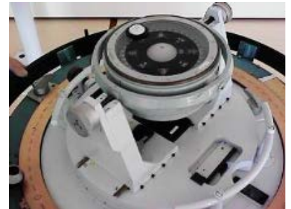
Magnetic compass undergoing test on our unique test stands
