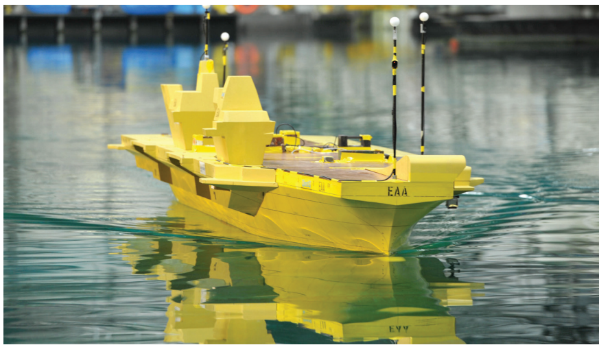
Model of Queen Elizabeth Class aircraft carrier operating in Ocean Basin (image reproduced courtesy of the Ministry of Defence)
