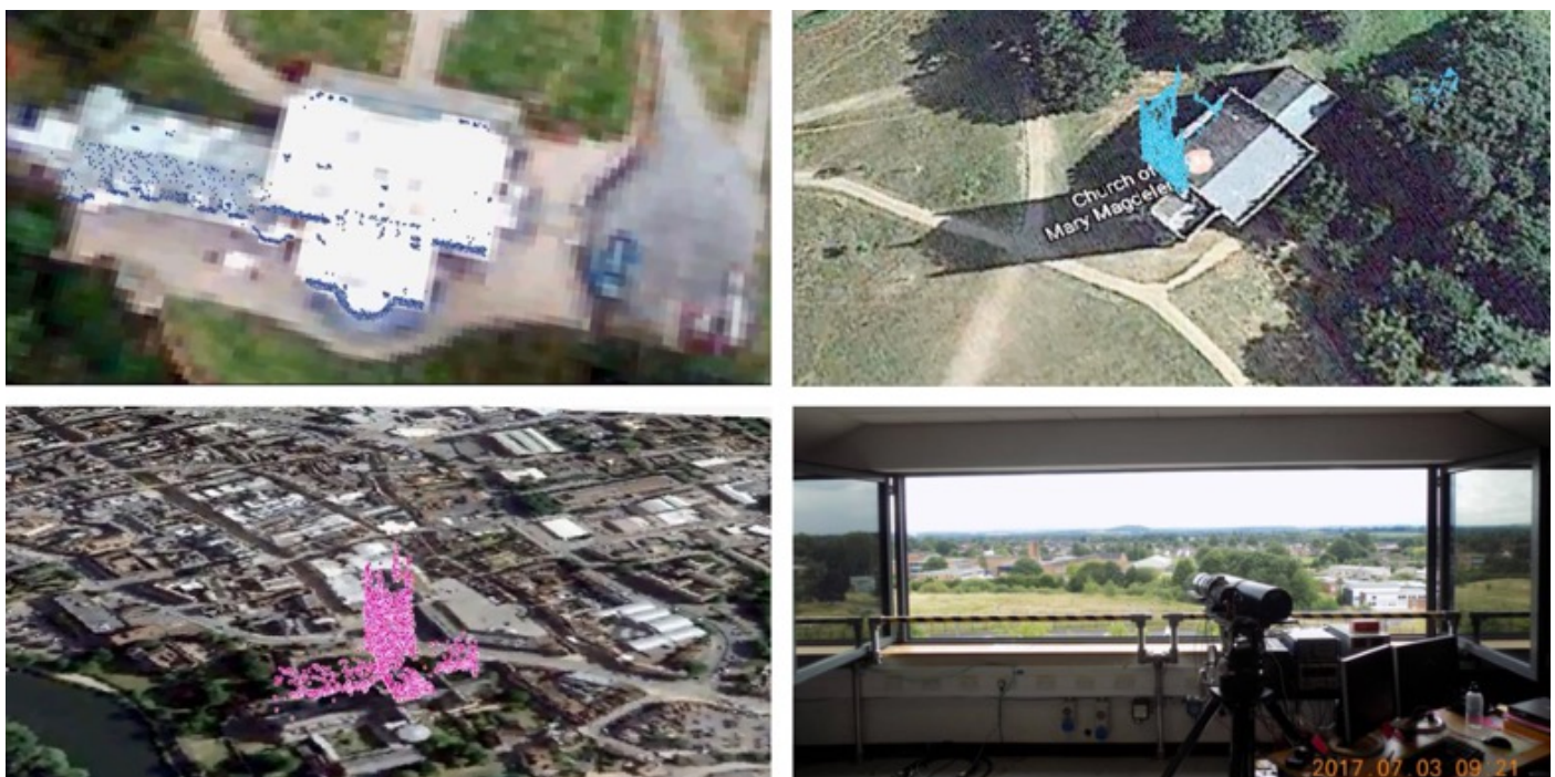
Figure 2: SDML 3D images (point clouds) of Targets of Opportunity. Top left: Severn Bank House (7.6 km). Top right: Croome Church (10.1 km). Bottom left: Worcester Cathedral (11.6 km). At our scaled-down power-aperture product, a 10 km target gives a photon flux at the receiver equivalent to 30 km slant range from a HAPS deployed at 23 km (75 kft) altitude. Bottom right: SDML equipment. (Satellite imagery: Google.)
