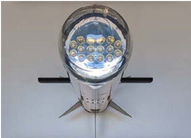
Self-contained target towed by a host aircraft
