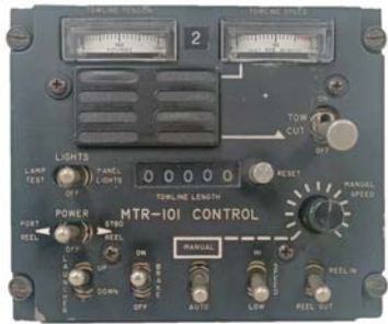
The Operator Control Panel, provides the user with readouts including towline reeling speed, tension, status indicator lights and function control switches.
