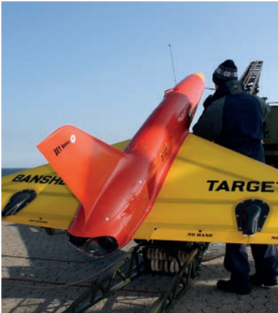
The Banshee target can simulate an enemy aircraft or cruise missile
