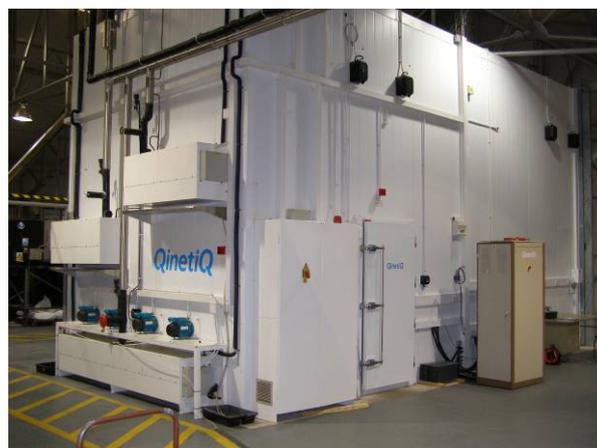
*The small chamber offers faster heating/cooling times and a cost effective option for smaller test items*
