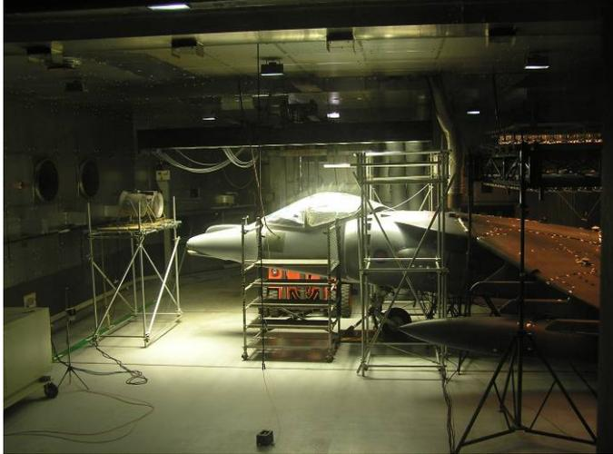
*A temperature range from +70°C to -70°C, and full humidity control, means the exact customer required scenario can be simulated.*
